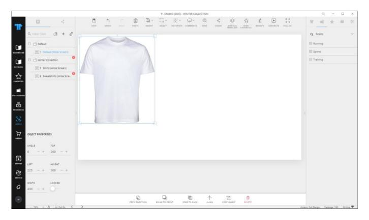
You can rotate the image by changing the angle using the (-) and (+) signs. You can resize the image by dragging any of its corners. To move the image, click it and drag to the desired location or change the values displayed in the "Top" and "Left" fields using the (-) and (+) signs. These values represent the distance of the object from the top left corner of the window.
