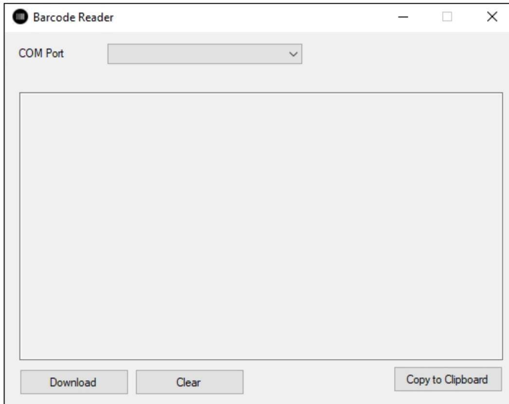
To scan the barcodes, attach the reader to your computer and select the port, if not selected by default. You can then click **Download** to load the scanned barcodes in the above window. To copy the barcodes, click **Copy to Clipboard**.
